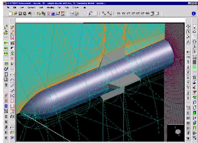
STORM is a 3D viscous flow solver that combines a strongly conservative finite-volume formulation with advanced physical modeling capabilities such as:
