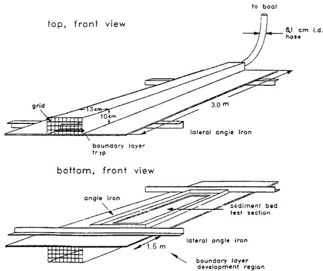
**Fig. 1.** Schematic of in situ straight flume (adapted from Ravens and Gshwend 1999)
