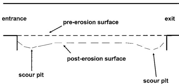
**Fig. 2.** Schematic of flume test section (side view) showing pre- and post-erosion sediment surfaces and location of scour pits
