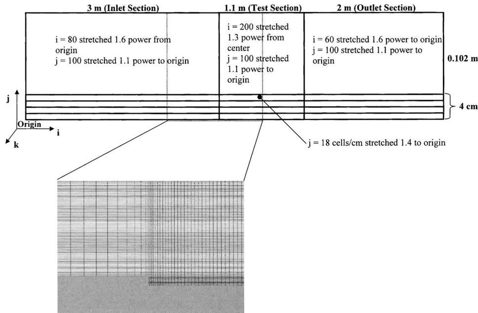
Fig. 3. Geometry and grid used in modeling study (figure is not to scale)
