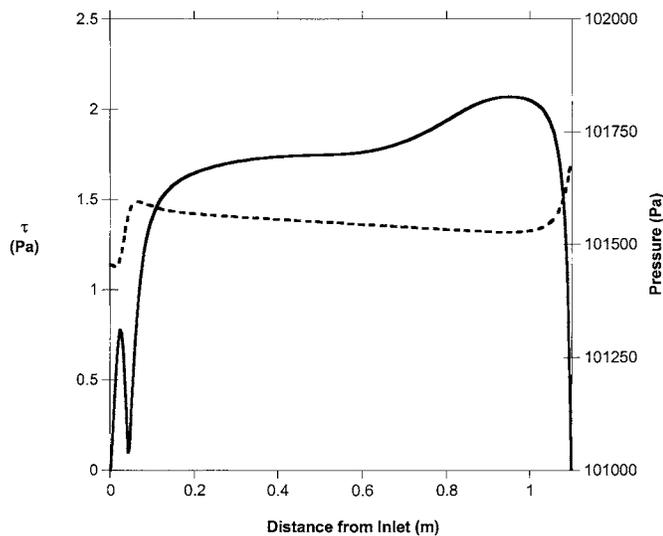
Fig. 4. Model-calculated bottom shear stress (—) and pressure (---) for 1 cm erosion at 1 m/s average flow velocity
