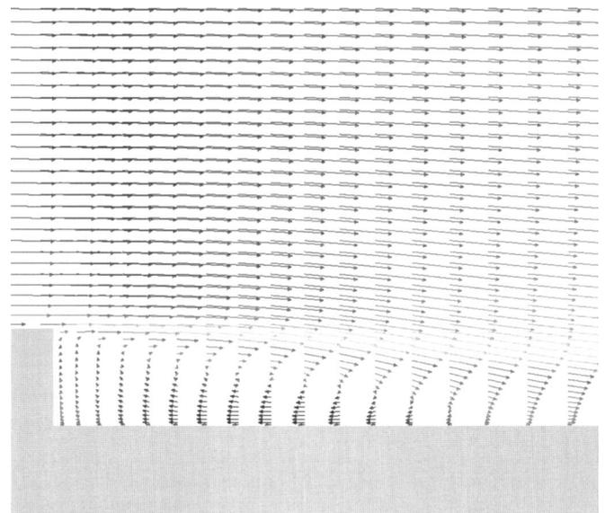
Fig. 5. Blowup of test section inlet. Circulation cell shown by velocity vectors for 2 cm erosion at 1 m/s average flow velocity.
