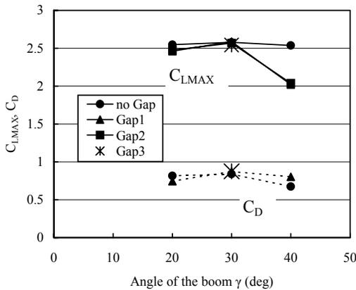
Fig.15 Effect of the boom angle and the gap width on  $C_{LMAX}$  and  $C_D$  at  $C_{LMAX}$  ( $AR=2.63, \beta=35deg$ )
