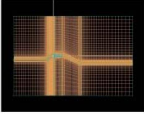
Fig.17 Grid example of the calculation on the hybrid sail (AR=2.34,  $\beta=35\text{deg}$ ,  $\gamma=20\text{deg}$ )
