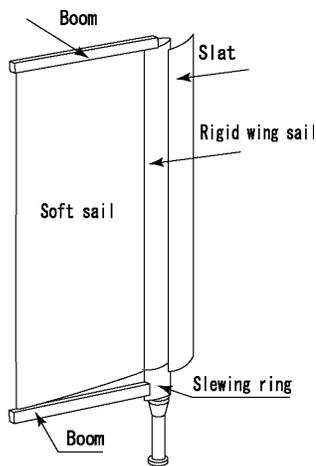
Fig.3 Basic concept of the high performance hybrid-sail
