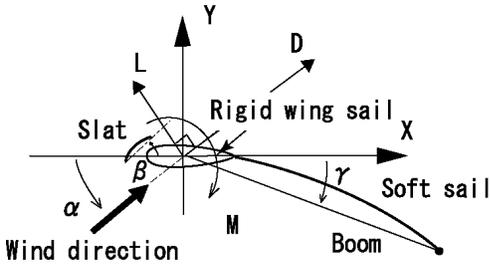
Fig.6 Coordinate system and definitions
