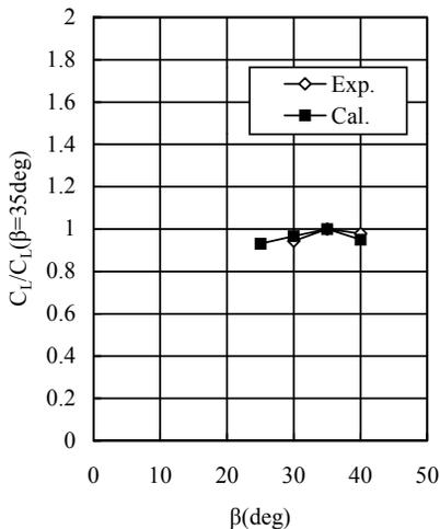
Fig.20 Comparison between the calculation results and the experimental ones on relative  $C_L$  when the slat angle is change (AR=2.34,  $\alpha=20\text{deg}$ ,  $\gamma=30\text{deg}$ )
