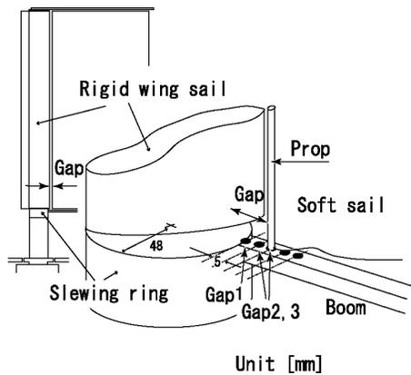
Fig.14 Hybrid-sail with the gap between the rigid wing sail and the soft sail, and position of the prop in the soft sail
