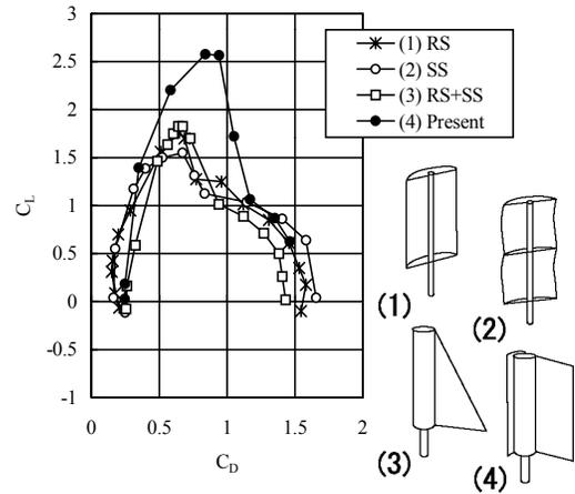
Fig.12  $C_L$ - $C_D$  curve on the present hybrid sail ( $AR=2.63$ ) and the previous sails (Ishihara,1980)(RS; Rigid Sail, SS; Soft Sail)
