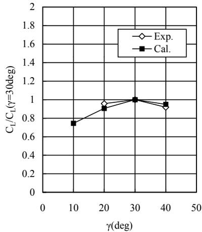
Fig.19 Comparison between the calculation results and the experimental ones on relative  $C_L$  when the boom angle is change (AR=2.34,  $\alpha=20\text{deg}$ ,  $\beta=35\text{deg}$ )
