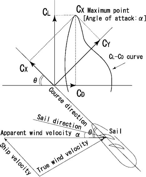
Fig.7 Relationship between the course direction of a ship and the thrust by the wind
