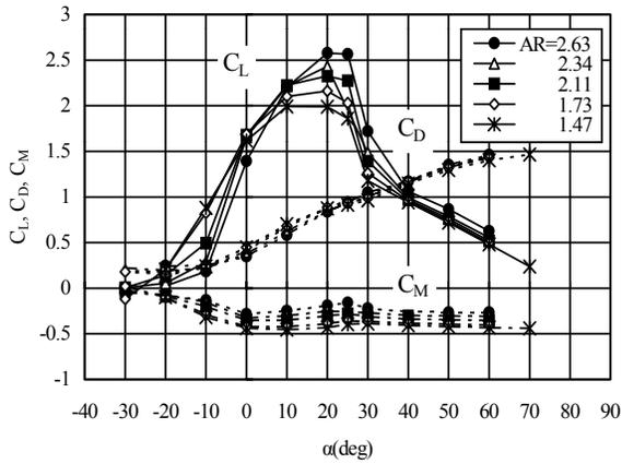
Fig.10 Aerodynamic characteristics of the hybrid sails in the difference of the aspect ratios ( $\beta=35\text{deg}$ ,  $\gamma=30\text{deg}$ )
