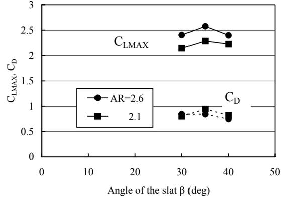
Fig.8 Effect of the slat angle on  $C_{LMAX}$  and  $C_D$  at  $C_{LMAX}$  ( $\gamma=30deg$ )
