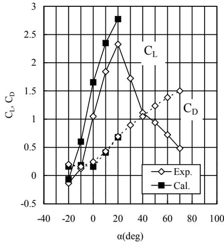
Fig.18 Aerodynamic characteristics of the hybrid sails comparing the calculation results with the experimental ones (AR=2.34,  $\beta=35\text{deg}$ ,  $\gamma=20\text{deg}$ )
