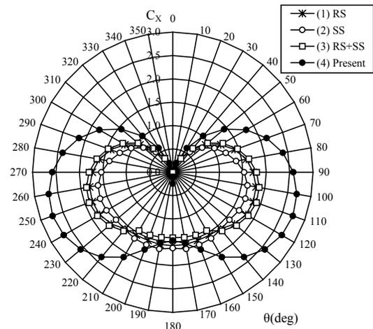
Fig.13 Polar curve on  $C_X$  (RS; Rigid Sail, SS; Soft Sail)
