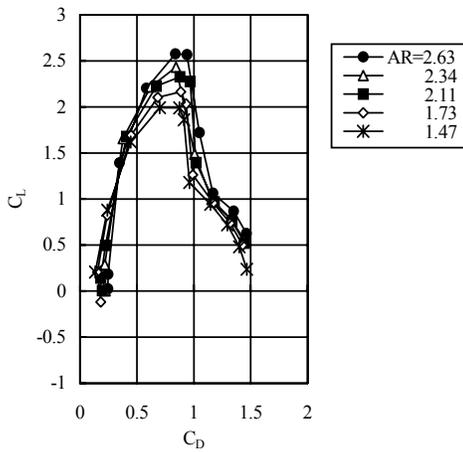
Fig.11  $C_L$ - $C_D$  curve of the hybrid sails ( $\beta=35\text{deg}$ ,  $\gamma=30\text{deg}$ )
