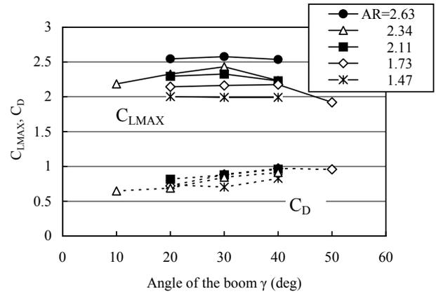
Fig.9 Effect of the boom angle and the aspect ratio on  $C_{LMAX}$  and  $C_D$  at  $C_{LMAX}$  ( $\beta=35deg$ )
