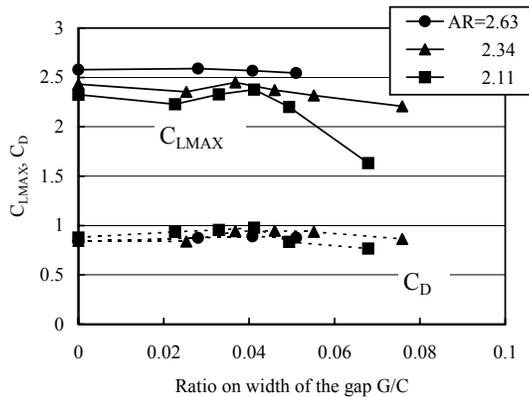
Fig.16 Effect of the gap width and the AR on  $C_{LMAX}$  and  $C_D$  at  $C_{LMAX}$  ( $\beta=35deg, \gamma=30deg$ )
